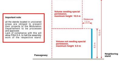
Plan of lateral elevation
